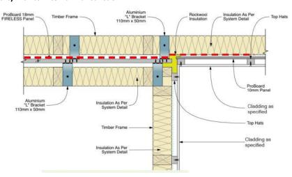
Where two party walls meet perpendicularly, it is proposed for the corner of the walls to be additionally fixed with an aluminium angle either on the inside or outside faces of the corner as shown. The 18 mm ProBoard panel is still to be fixed to the timber frame with aluminium angle with minimum dimensions of the tested system.
